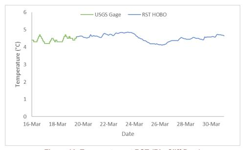
Figure 16. Temperature at RST (Big Cliff Dam)
